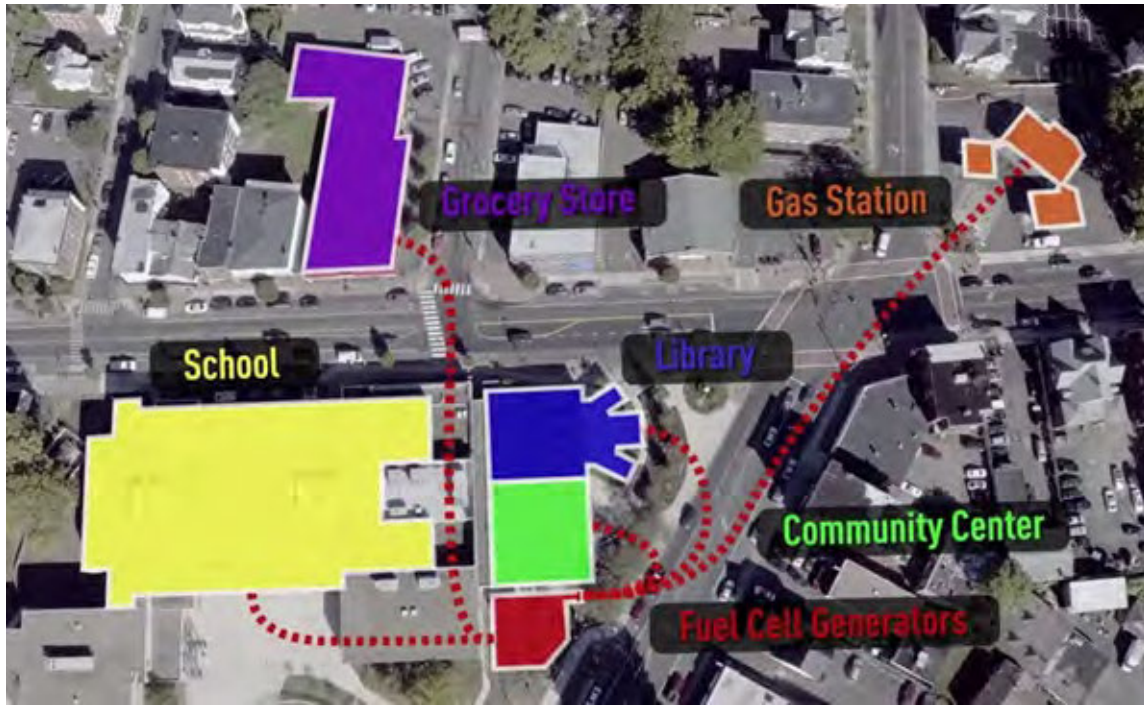
Figure 15 ■ Fuel cell-based microgrid supplying energy to key community locations (Constellation Energy)
